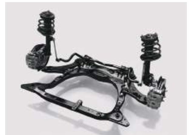
The Front Suspension Uses TNGA-Specific Macpherson Struts.
